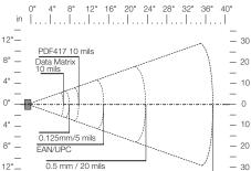
\* The reading distances for each scanner are typical distances measured from the front end of the scanner bezel in an office environment (200 lux) with extended reading range activated.
